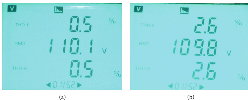
FIGURE 20: Experimental THD in linear load (a) and nonlinear load (b).
